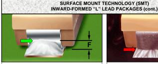
ACCEPTABLE MINIMUM HEEL FILLET HEIGHT (F) The heel fillet height (F) shall be sufficient to
